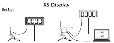
Plug the *XS Display* into the *Timer* or into the *USB Interface* when connected to a computer. The time of the finished skier will display for 10 seconds, then clear to 00.00, or be replaced with a new time.
