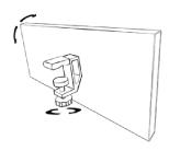
The included mounting clamp attaches to the back of the *TC-Display* and can be used as an adjustable tilt stand.
