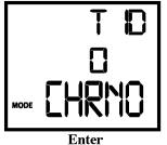
*Chrno* mode is the principal mode used for the majority of timing applications. When powered on, the *TC-Timer* automatically enters this mode.
